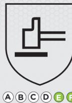
EN 388's testing method using only the Coup Test would at times result in two different gloves both having a cut level 5. However, after being tested with the ISO 13997 method where the TDM machine is used, the same gloves could score a cut level 5/C while the other an 5/E-a difference of up to 2000 grams of force! The new levels make it much easier to identify the different cut protection levels.
